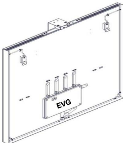
EVG for 2x LE When an EVG box has two connections it is not possible to adjust just one lamp. This box always needs two lamps to be fixed.
