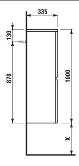
X =The exact height must be set during installation.
